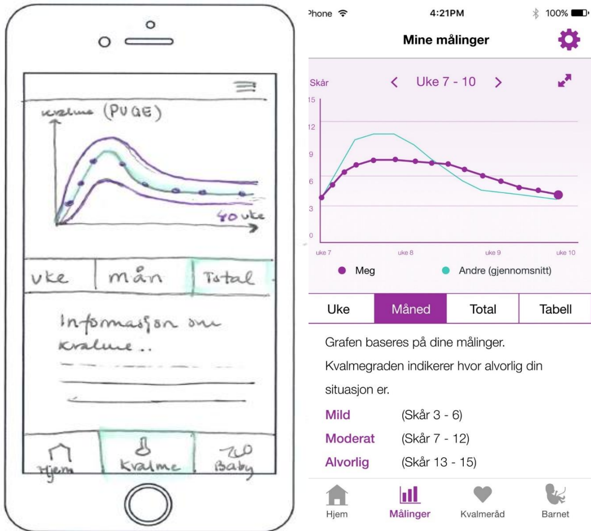
Figure 3.4: Overview of the women's logged PUQE score (purple graph) compared to the mean PUQE score of other pregnant women (blue graph) displayed as a graph. The illustration to the left is our sketch of the app, while the illustration to the right shows how the vision turned out after the app was developed.
